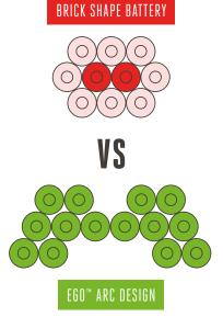
To achieve the desired voltage and amp hours needed for grounds maintenance equipment, several smaller lithium-ion cells are brought together into a single pack.
